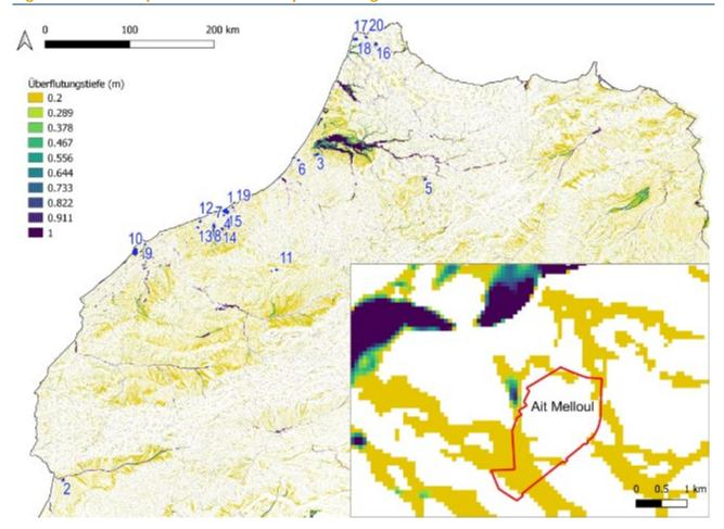
Figure 15 Flood depth in a one-hundred-year flooding scenario
