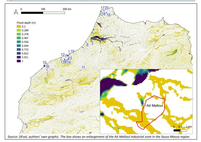
Figure 10 Flood depth in a one-hundred-year flooding scenario
